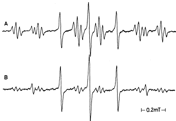
Fig. 1. ESR signal recorded during photolysis of p -benzoquinone in ethanol flowing at a resident time of 0.5 s at 293 K. Concentration of quinone, (A) 10 and (B) 1.0 mmol dm ^{-3} .
